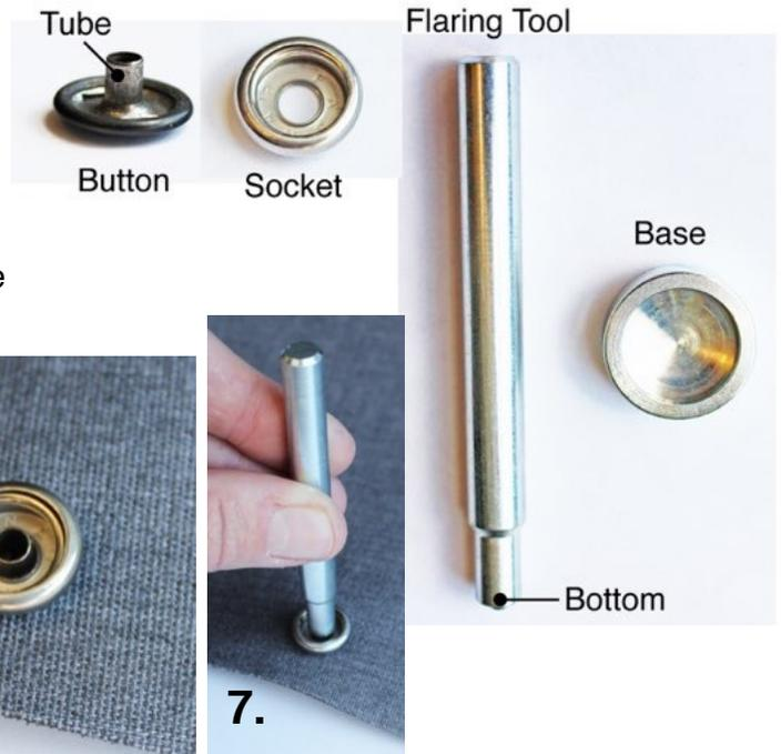
6. Place the Socket onto the Tube with the ring of the Socket facing up.
