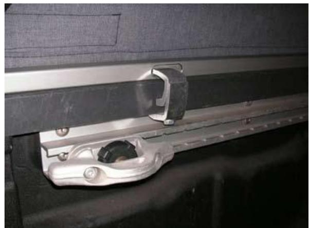
Tighten down firmly...don't over-tighten. Just make sure they are snug so the Softopper bedrail is unable to move.
