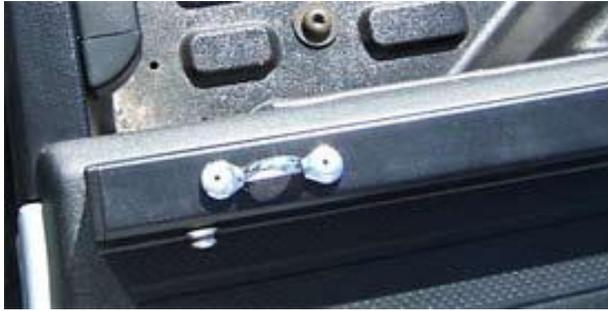
It can be placed evenly with the inside edge of the truck's side rail or moved outward slightly. It is recommended that it rests within ½ inch from the inside.
