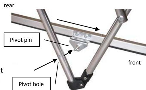
**NOTE:** The pivot pin is designed to loosen slightly to allow for movement and flexing of the truck bed.
