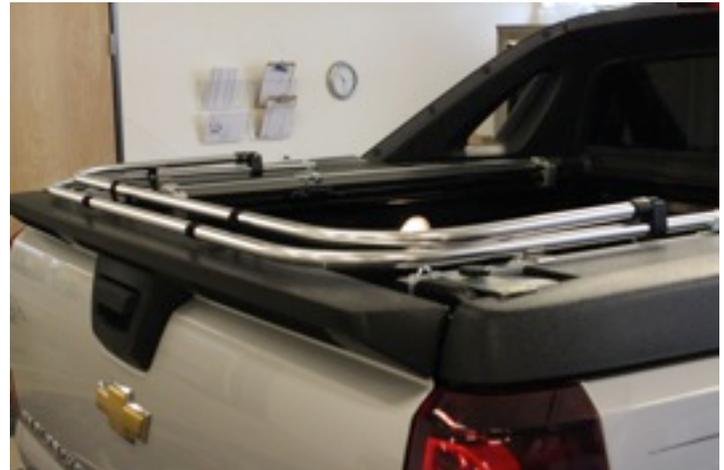
**Step 5** Install the bulb seal. Clean the area under the side toolbox door with a rag or similar. Peel the red backing off of the bulb seal and install it centered in front of the tool box opening. NOTE: The flange on the bulb seal should be snug up against the toolbox. **See photo.**
