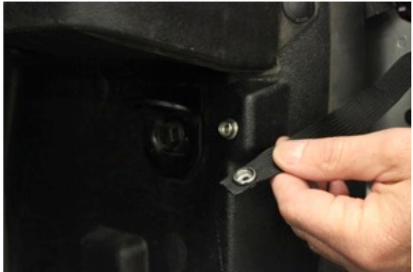
**Step 7B- For 2001 to 2006 models only.** Install the two short webbing straps with the small loop onto the longer webbing straps that are sewn into the lower inside rear of the canopy. Slide the small loop over the prong on the hinged tie down part on the rear ends of the bed. **See photo.** While pulling rearward on the lower side of the canopy pull the tail on the strap until the side is snug and showing minimal wrinkles.
