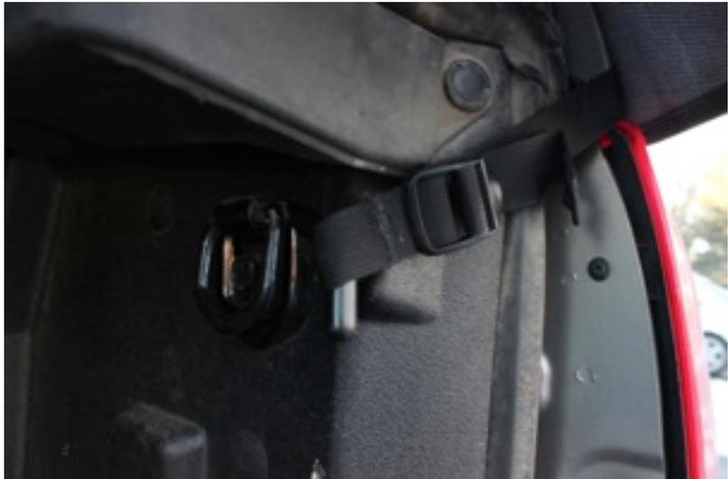
**Step 8** Install in the rear window panel. Climb into the bed of the truck or sit on the tailgate with the rear window panel in hand. Locate the center of the rear cross by the middle snap and line up the middle of the rear window panel which has a hole punched dead center. Press the hook and loop together evenly. Attach the side zippers at the top and attach the small hook and loop flaps. These flaps just help to keep the zippers from coming off unintentionally when opening the rear panel.
