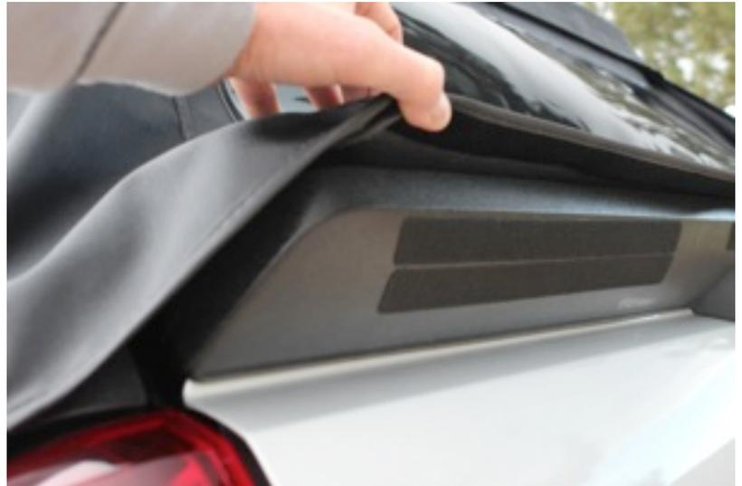
**Note regarding accessing your side toolboxes.** The Softopper framework does not allow the box covers to open past 90 degrees. Use caution when reaching into the toolbox, and hold the box door open, as it can slam down on your fingers!
