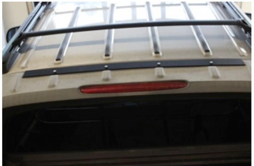
**Step 2** Using the Torx T-30 key or driver remove the T-6 bolt from each of the black triangular parts at the rear of the vehicles box. Keep the long bolts in a safe place along with the 4 other bolts. Install the 2 black plates loosely using the 2- 80mm bolts with plastic turn knobs and 2 small washers. **See photos.**
